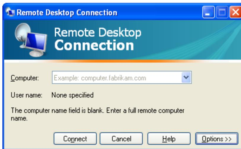
In the "Computer" field, you will type in the name of your office computer which you should have already obtained. Type the fully qualified domain name to be sure you are connecting to the correct computer. The fully qualified domain name is the name of the machine
