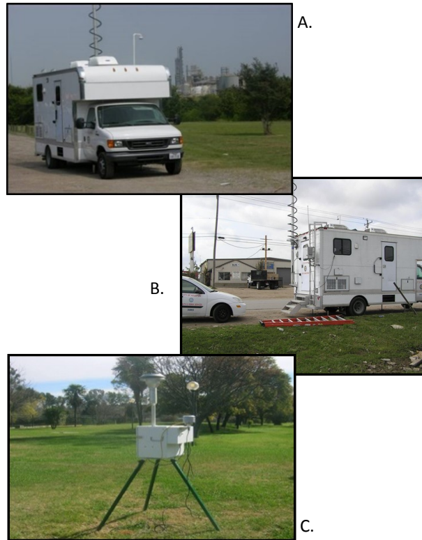
Photos: Mobile Ambient Air Monitoring Laboratory—MAAML (A and B) and a tripod-mounted inhalable particle air sampler (C)
