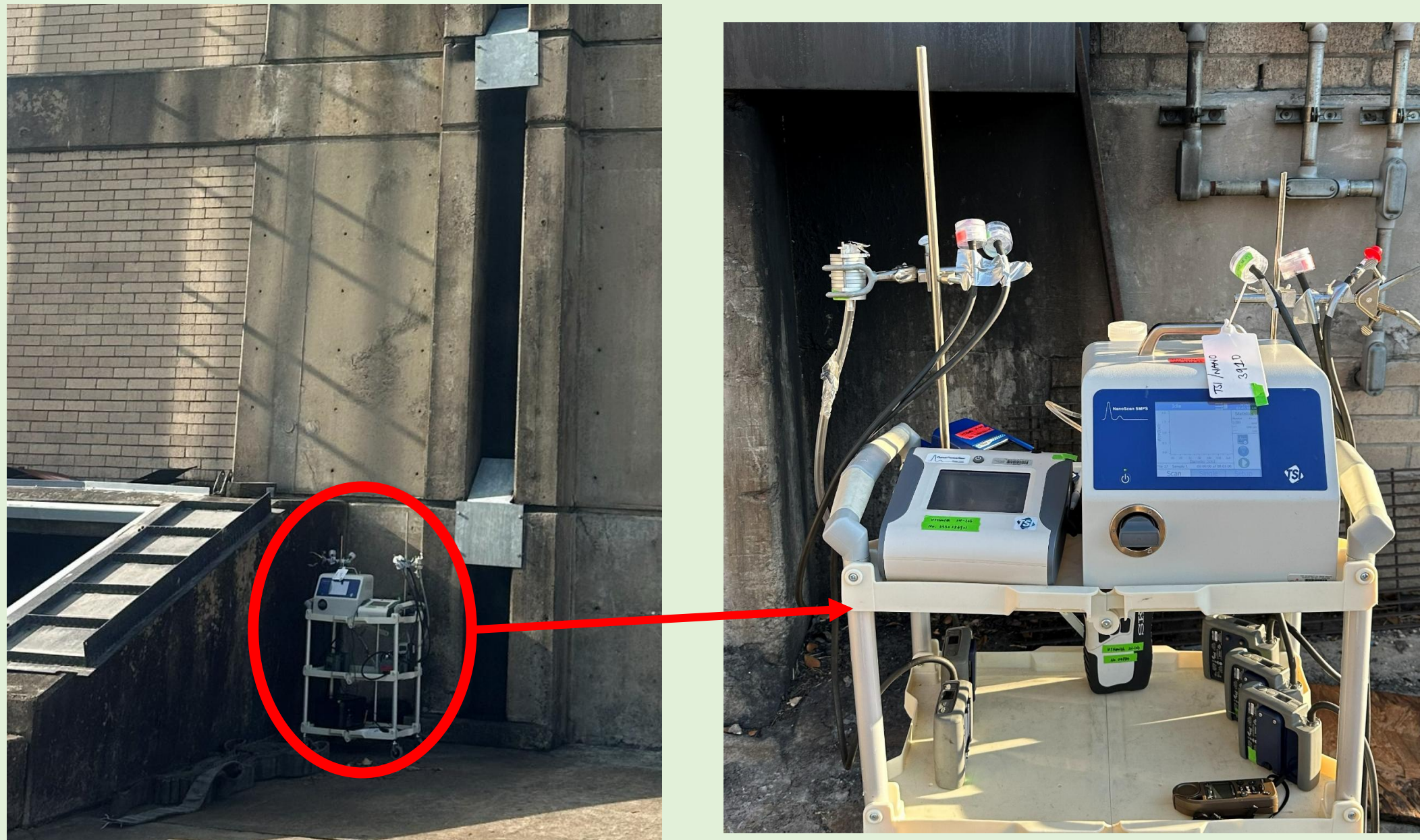
Figure 4. Outdoor: Direct-reading real-time instruments. The location was selected with the on-site HFD commander to minimize training disruption and identify the downwind direction.
