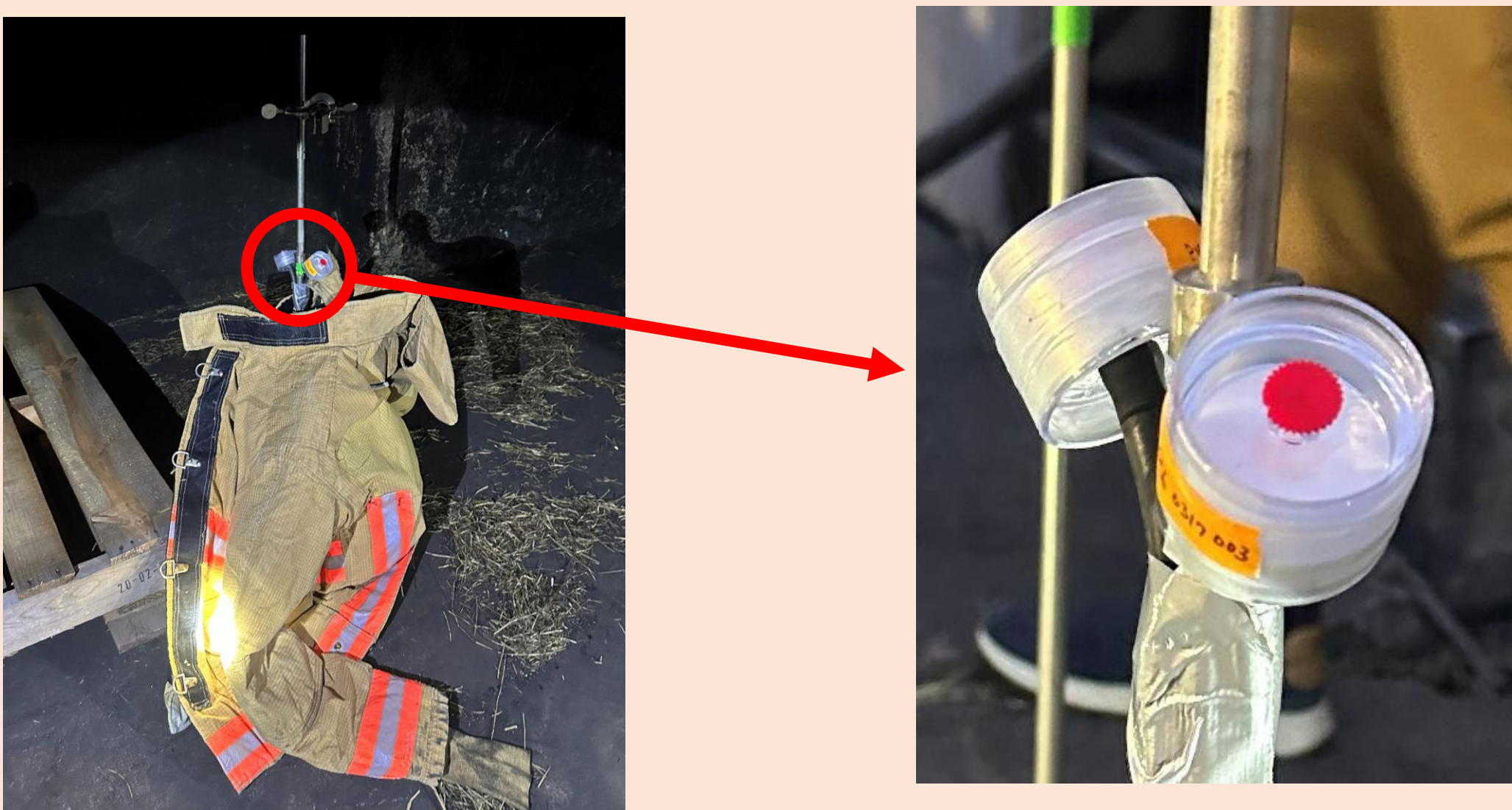
Figure 5. Indoor: Mixed Cellulose Ester (MCE) membrane samplers. The stations were positioned approximately 200–250 cm from the fire source. Each sampler was covered with turnout gear to protect it from high temperatures.
